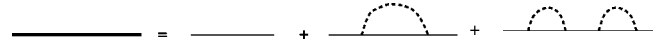
FIG. 5. A diagrammatic depiction of the approximation used in the calculation. The thick line indicates \hat{G} . The first term on the right-hand side of the equation refers to \hat{G}_0 . The second term refers to the exchange -like diagram referred to in the text. The final term is the second order correction.
